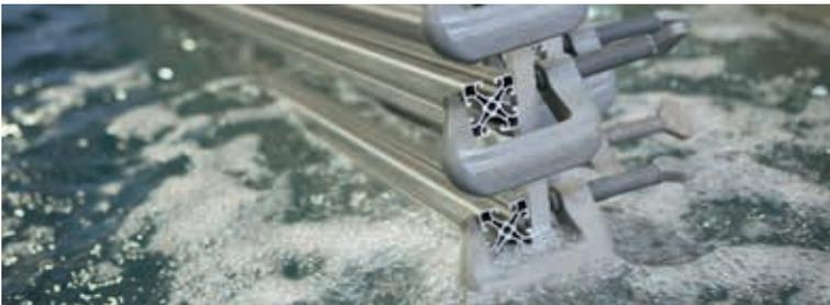
Eloxal coats the aluminum with an oxide layer, both to increase the resistance of the aluminum's surface to weather conditions and provide an extremely hard surface wear resistant surface to use.
